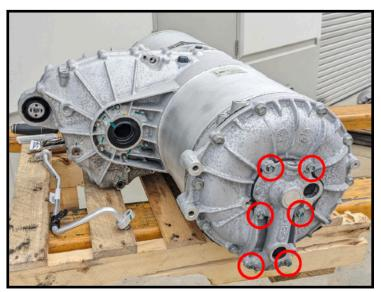
Remove the six 10mm bolts securing the rotor seal manifold.
