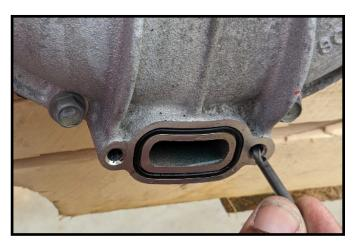
Apply a thin bead of silicone sealant around the new Rotor Seal Bypass Manifold as shown. Apply a thin film of o-ring grease to the new Rotor Seal Bypass Manifold as shown.
