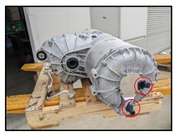
Take the o-ring from the external coolant line and install it on the new block-off piece. Apply a small amount of o-ring grease to the o-ring. Install the block-off piece as shown and torque the bolt to 8Nm. Ensure the black AN cap is torqued appropriately.
