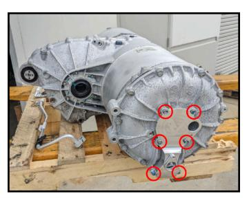
Apply a small amount of o-ring grease to the encoder and water fitting o-rings and install them in the new Rotor Seal Bypass Manifold. Torque the bolts to 8Nm.
